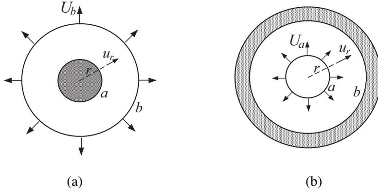
Figure 2: Radial loading of a hollow circular cylinder in which (a) the outer boundary  $r = b$  is given an outward radial displacement  $U_b$  while the inner bonded cylinder is kept fixed, and (b) the inner boundary  $r = a$  is given an outward radial displacement  $U_a$  while the outer casing is fixed. The radial displacement at an arbitrary  $r$  is denoted by  $u_r = u_r(r)$ .
