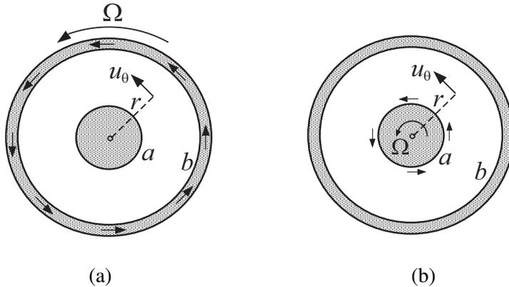
Figure 1: Azimuthal shear of a hollow circular cylinder in which (a) the outer bonded casing is given a rotation  $\Omega$  while the inner bonded cylinder is kept fixed, and (b) the inner cylinder is given a rotation  $\Omega$  while the outer casing is fixed. The inner and outer radii of the hollow cylinder are  $a$  and  $b$ , and  $u_\theta = u_\theta(r)$  is the circumferential displacement.
