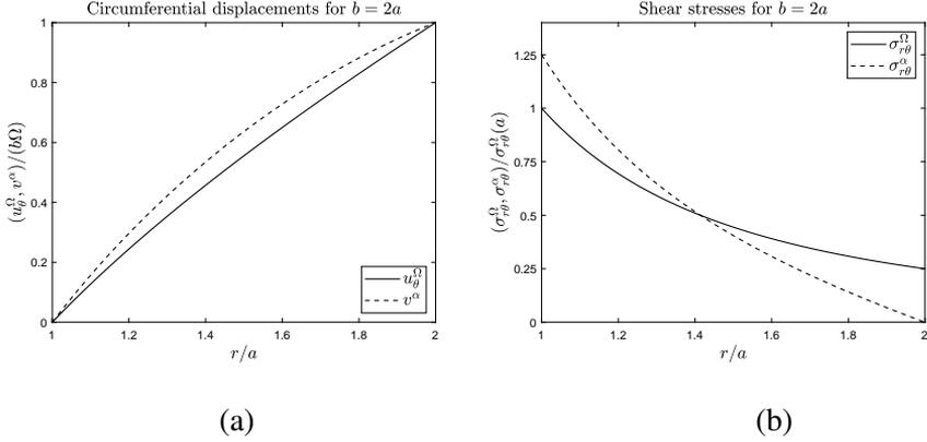
Figure 3: (a) The normalized displacements due to azimuthal shear  $\Omega$  and angular acceleration  $\alpha$  of a thin disk vs.  $r/a$ , in the case when  $\alpha$  and  $\Omega$  are related by the condition  $u_\theta^\Omega(b) = v^\alpha(b)$ . (b) The corresponding variations of the normalized shear stresses.
